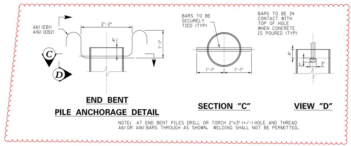
**END BENT PILE ANCHORAGE DETAIL**
