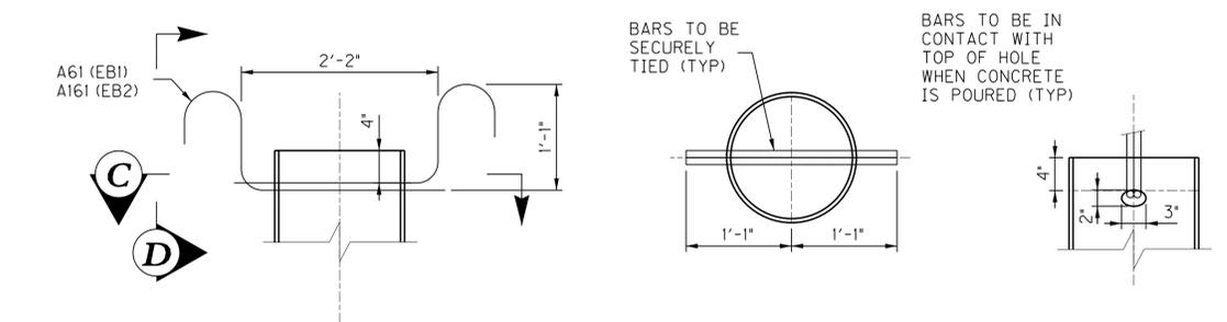
**END BENT PILE ANCHORAGE DETAIL**
