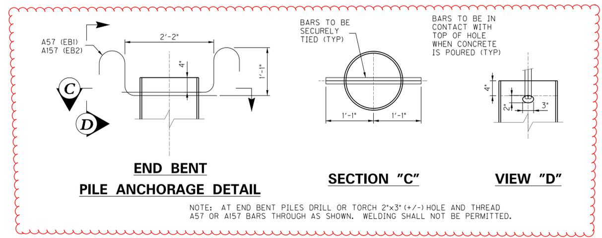
**END BENT PILE ANCHORAGE DETAIL**
