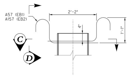
**END BENT PILE ANCHORAGE DETAIL**
